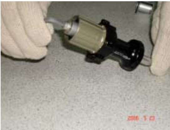
Step 2 Turn the wrenches in a counter clockwise direction to loosen the alloy cap
