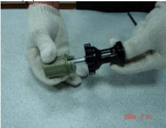
Step 4 With the 5mm allen wrench loosen the nut on the non-drive side and then remove it. Push the axle thru the hub body & detach the cassette body and spacer from the axle (see photo 5.1)
