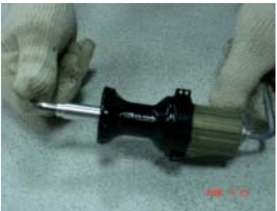
Step 7 Place the 5mm allen wrenches on the alloy cap side and turn clock wise to tighten
