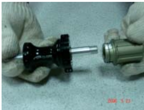
Step 4 Thread the cassette body onto the axle being careful to properly seat it onto the hub shell. Hold the left side of the axle and tighten clockwise
