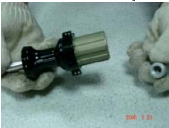
Step 6 Place the alloy cap over the axle and tighten (see photo 6.1)
