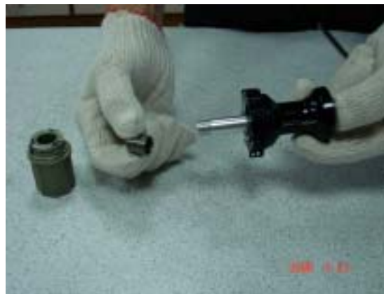
Step 4 With the 5mm allen wrench loosen the nut on the non-drive side and then remove it. Push the axle thru the hub body & detach the cassette body and spacer from the axle (see photo 5.1)
