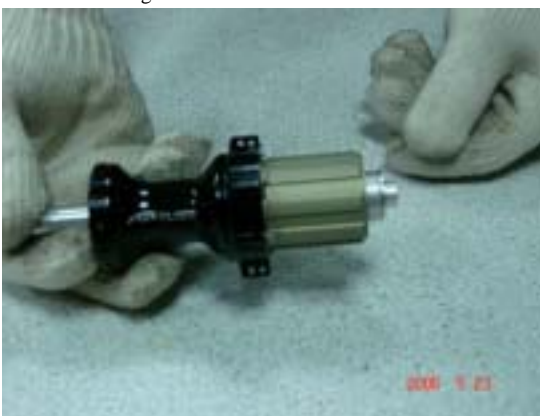
Step 5 Test to make sure the cassette body rotates freely on the hub/axle/bearings.
