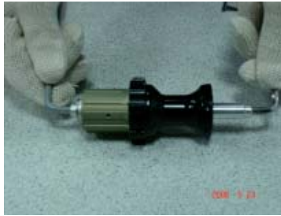
Step 1 Place a 5mm allen wrench into the stop nut of the cassette body and into the hollow axle on the non-drive side (see photo 1.1)
