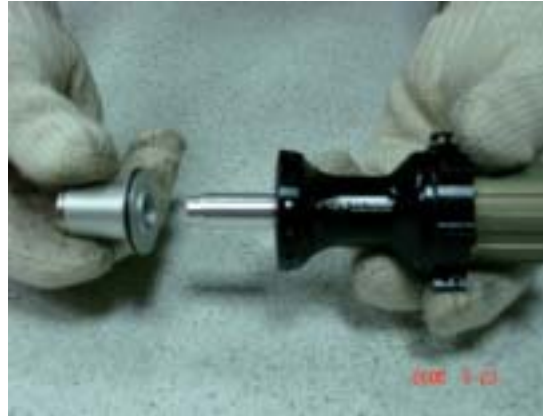
Step 10 Insert the LH alloy cap onto the axle and tighten
