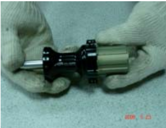
Step 5 Test to make sure the cassette body rotates freely on the hub/axle/bearings.
