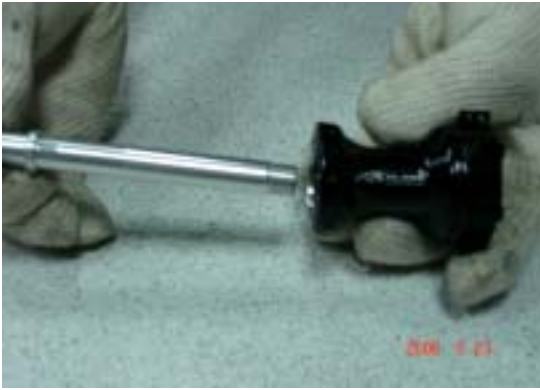
Step 1 Insert the axle into the hub body making sure that the threaded end goes into the hub
